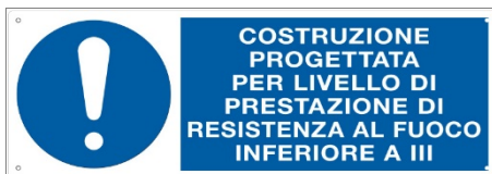
Image 15: Example of a signal for a fire resistance performance level lower than III
